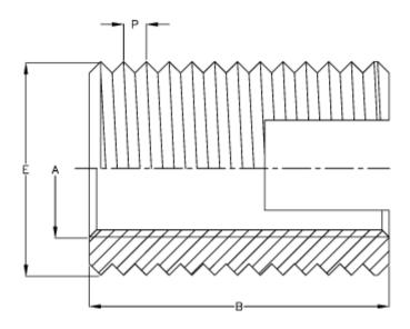
Female thread A = M18 Length B = 24 Male thread E = 22.0 Min hole depth blind hole = 29
